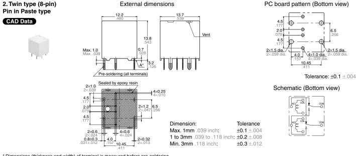
\* Dimensions (thickness and width) of terminal is measured before pre-soldering. Intervals between terminals is measured at A surface level.
