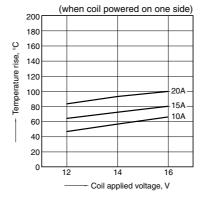
1.-(5) Coil temperature rise (at room temperature)
