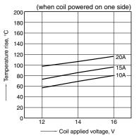
Measured portion: Inside the coil Contact carrying current: 10A, 15A, 20A Ambient temperature: 85°C 185°F
