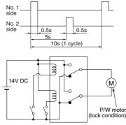
Load current waveform Current value: 25A
