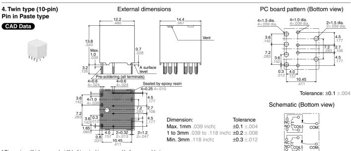
\* Dimensions (thickness and width) of terminal is measured before pre-soldering Intervals between terminals is measured at A surface level.
