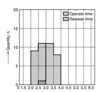
5-(1). Electrical life test (at rated load)
