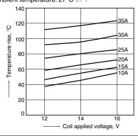
1-(2). Coil temperature rise Sample : CP1H-12V, 3pcs Point measured : Inside the coil Ambient temperature: 85°C 185°F
