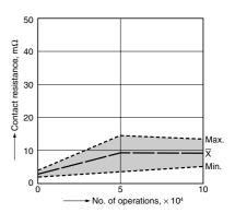
5-(2). Electrical life test (at capacitor load)
