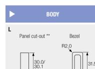
Cut-outs must be punched in the direction of insertion
