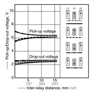
4-(2) Influence of adjacent mounting Tested sample: DS2Y-S-DC12V, 10 pcs. Ambient temperature: 20°C 68°F
