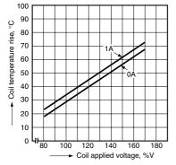
(200 mW Standard type) Tested sample: HY1Z-12V, 5 pcs. Ambient temperature: 23°C 74°F
