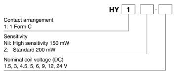
Note: In case of 5 V drive circuit, it is recommended to use 4.5 V type relay.
